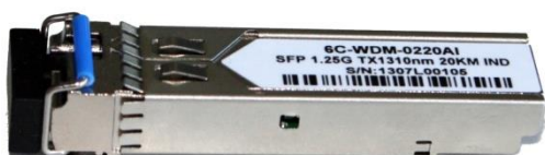
1000Base-BX WDM Singlemode (TX 1310 nm – RX 1550 nm)
