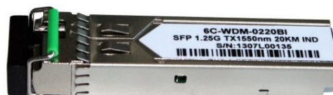
1000Base-BX WDM Singlemode (TX 1550 nm – RX 1310 nm)
