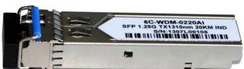
1000Base-BX WDM Singlemode (TX 1310 nm – RX 1550 nm)
